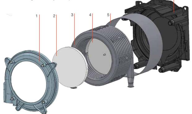
The metallic disk separates the combustion chamber and the condensing part and the disk position is variable: this distinctive features guarantees an optimized condensing heat exchange for each specific power size.
